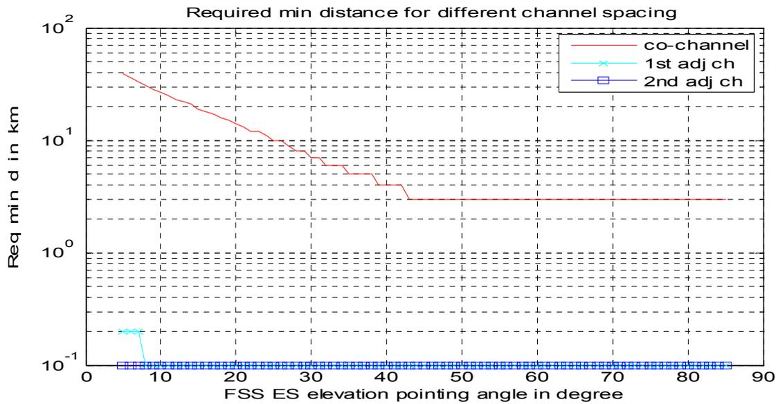
The following figure shows the minimum required distance in km between BWA urban BS with Scenario 2 ACLR values and 8 m FSS ES with 5° to 85° elevation pointing direction.
