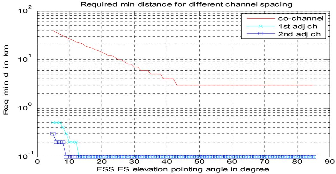
Note that distances below 100 m are not considered in the calculation of required separation distances.
