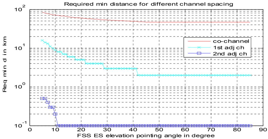
The following figure shows the minimum required distance in km between BWA urban BS with Scenario 2 ACLR values and 32 m FSS ES with 5° to 85° elevation pointing direction.
