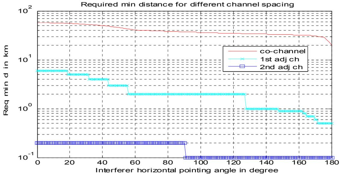
The following three figures show the minimum required distance in km between BWA rural BS with Scenario 2 ACLR values and 8 m FSS ES with 5°, 25°, and 50° elevation pointing direction, respectively. The BS antenna horizontal pointing direction is from 0° to 180°.
