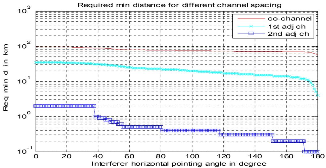
The following three figures show the minimum required distance in km between BWA rural BS with Scenario 2 ACLR values and 32 m FSS ES with 5°, 25°, and 50° elevation pointing direction, respectively. The BS antenna horizontal pointing direction is from 0° to 180°.
