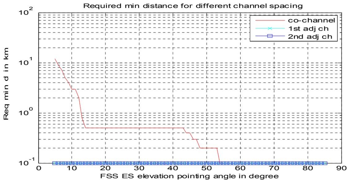
The following figure shows the minimum required distance in km between BWA urban BS with Scenario 2 ACLR values and 1.2 m FSS ES with 5° to 85° elevation pointing direction.
