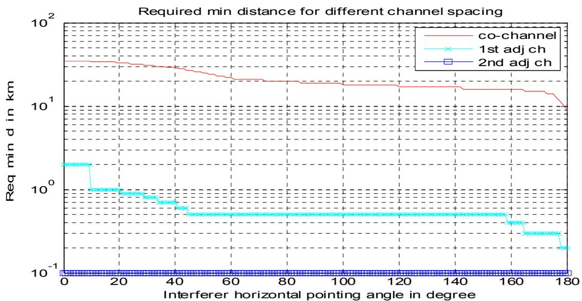
The following three figures show the minimum required distance in km between BWA rural BS with Scenario 2 ACLR values and 1.2 m FSS ES with 5°, 25°, and 50° elevation pointing direction, respectively. The BS antenna horizontal pointing direction is from 0° to 180°.
